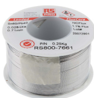
800-7661 0.71 mm solder wire, melting at: 183°C, composition: Sn 60%, Pb 40%, weight 250g
