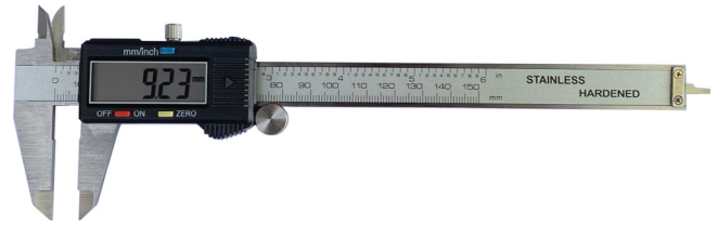
243-6615 150 mm digital calliper, imperial and metric reading, 0.03 mm accuracy
